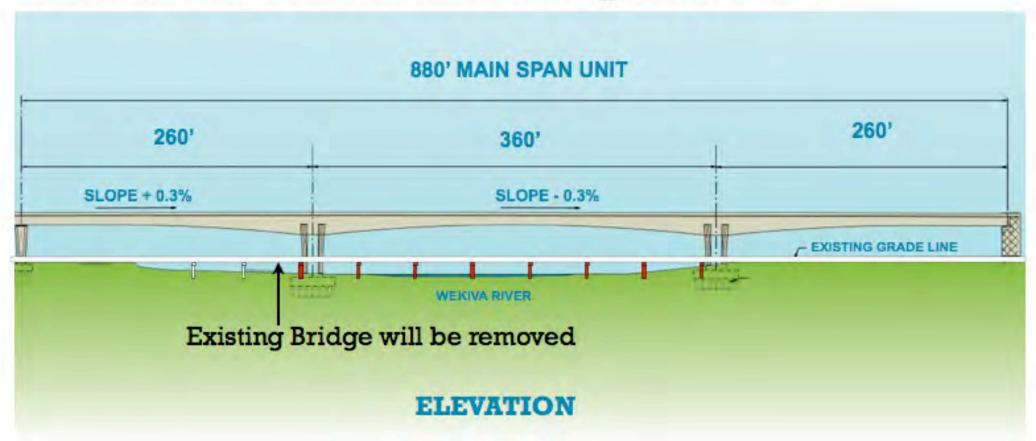
8 Piers of the existing bridge will be replaced with 1 span and 2 piers for the new bridge
